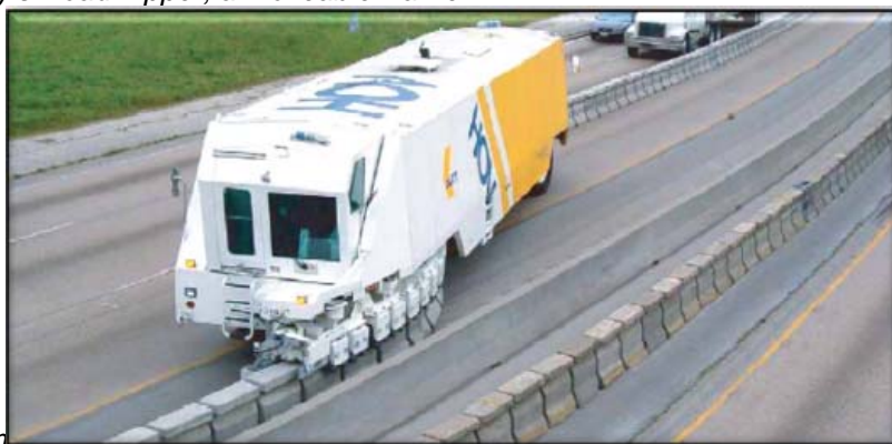
Lindsay's Road Zipper, a Moveable Barrier
